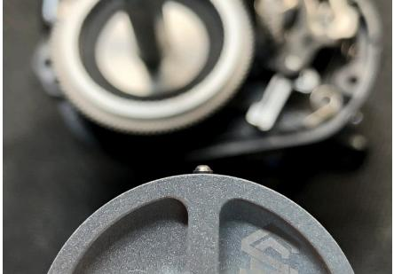
Insert spring and detent into the drag disk washer. The clicker has been tuned for the smoothest operation to audible sound.
