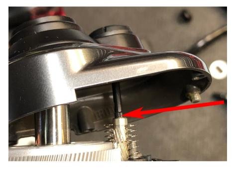
Note: When installing gear cover back on, make sure the spool tension shaft goes into pinion gear.
