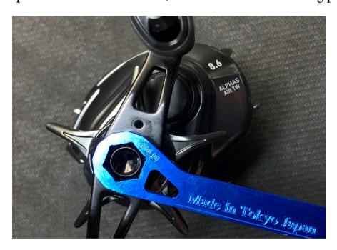
Remove the 10mm handle lock nut.
