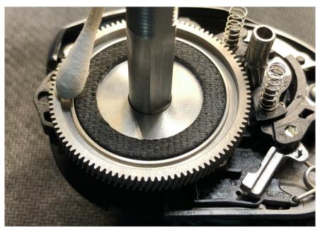
Apply degreaser to cotton swab and clean inside edge/inner ring of main gear where the "clicker ring" will sit. A tiny bit of super glue is needed to hold clicker securely in place. Clicker ring is precisely machined to have a perfect fit. \*Note: <u>DO NOT</u> test fit clicker ring! Can be hard to remove without damaging ring without proper tools.
