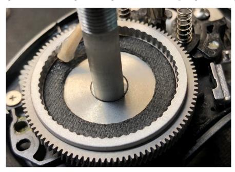
Install gear assembly into reel. Using the same grease you use on drag washer, apply a light layer on the inside of "Metal" clicker ring. \*NOTE\* PLASTIC CLICKER RING CAN BE RUN DRY FOR MAXIMUM AUDIBLE CLICKING SOUND.
