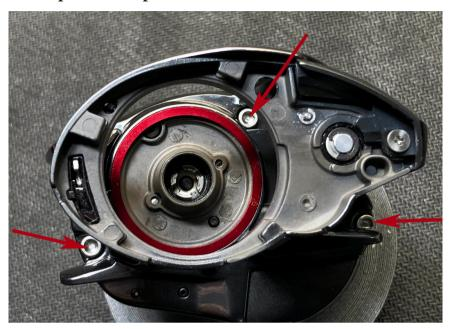
Remove 3 screws using 2.5mm allen wrench.
