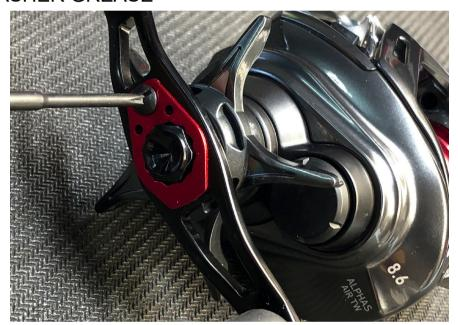
Using the phillips or flat head screwdriver, remove the handle locking plate.
